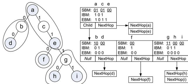
**Figure 1.** An SST with  $K=3$  and the corresponding data structure. The darker binary trie nodes represent valid prefixes.
