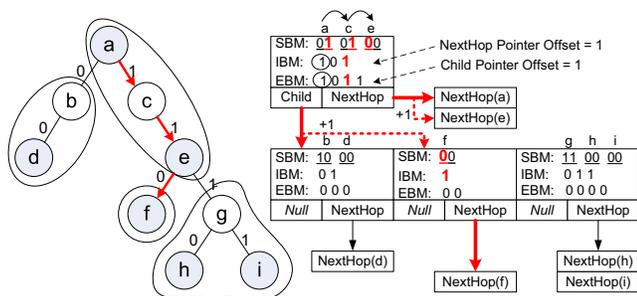
**Figure 2.** Assuming the IP address under lookup is “1100”. The first SST node lookup returns the child pointer and the best matched prefix so far; the second SST node lookup returns the best matched prefix.
