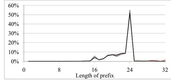
Figure 4: Prefix histogram of sample routing tables.
