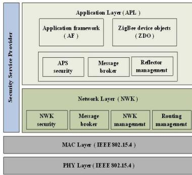
Fig. 1. Diagram of ZigBee stack.
