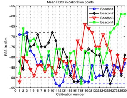
Fig. 13. Mean RSSI in calibration points .
