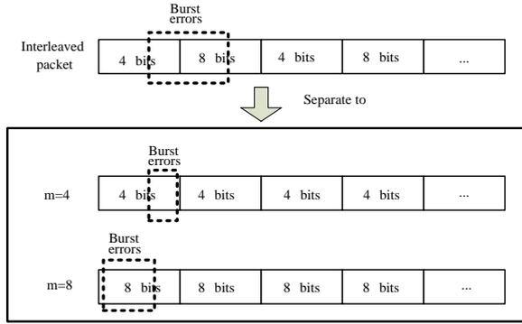
Figure 5. Burst errors dispersed on two symbols
