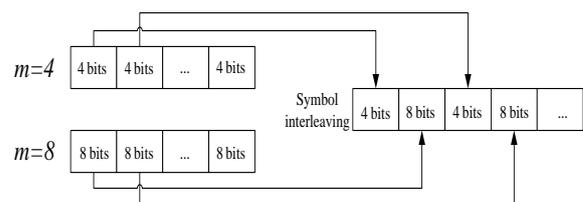
Figure 4. Packet interleaving on a symbol-by-symbol basis
