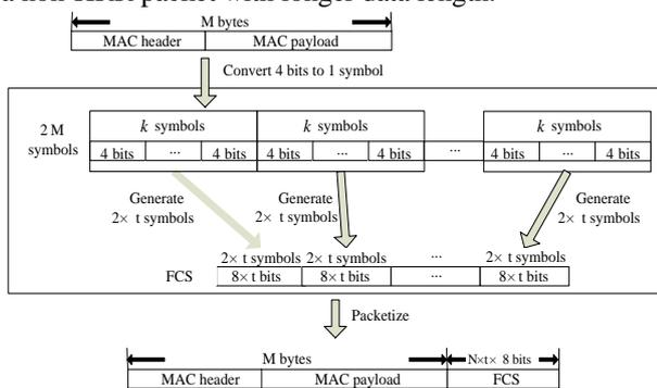
Figure 2. An HRR encoded with  $m = 4$
