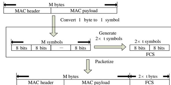
Figure 3. A non-HRR encoded with  $m = 8$
