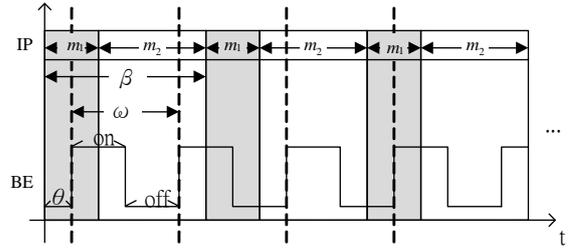
Figure 6. On-off bit error model
