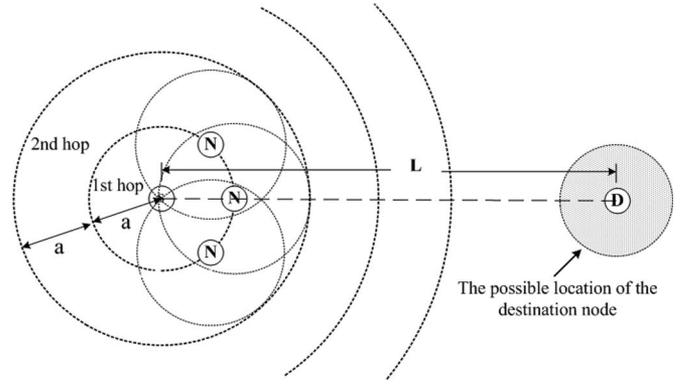
Fig. 1. Behavior of multihop packet forwarding via flooding in a dense mobile *ad hoc* network.
