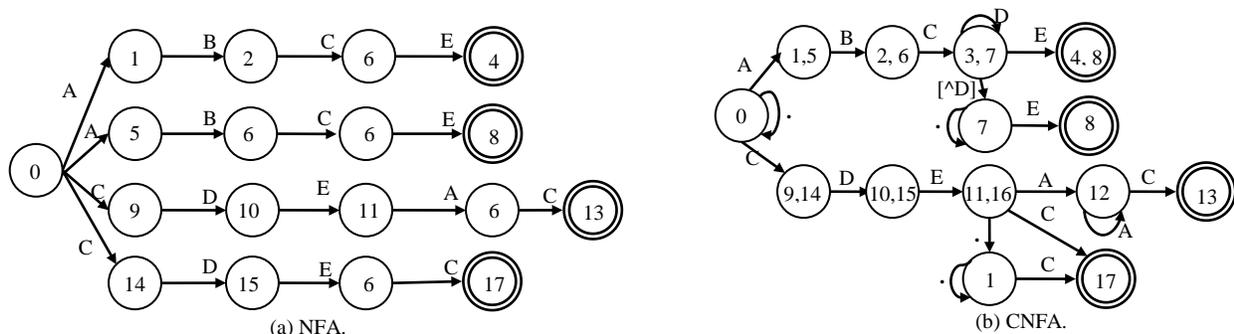
Figure 4. NFA and CNFA for Rule Set = {ABCD\*E, ABC.\*E, CDEA+C, CDE.\*C} and  $\Sigma = \{A, B, C, D, E\}$ .
