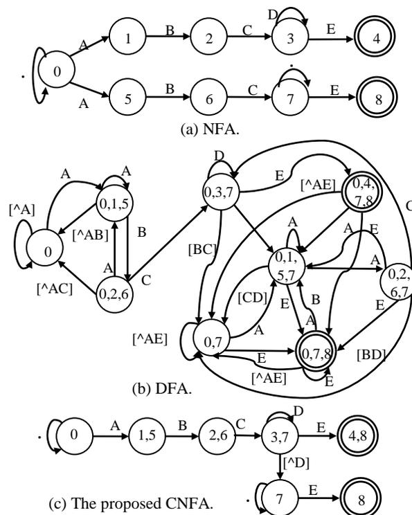
Figure 2. Finite State Automata for {ABCD\*E, ABC.\*E}.
