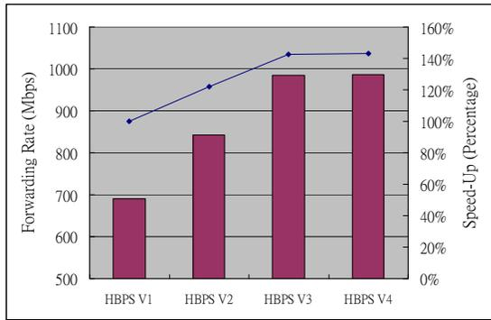
Figure 9. Forwarding rates and speed-ups.
