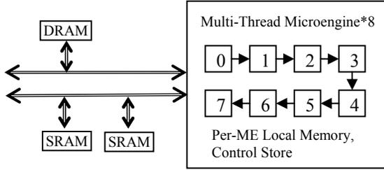
Figure 5. IXP2400 component diagram.
