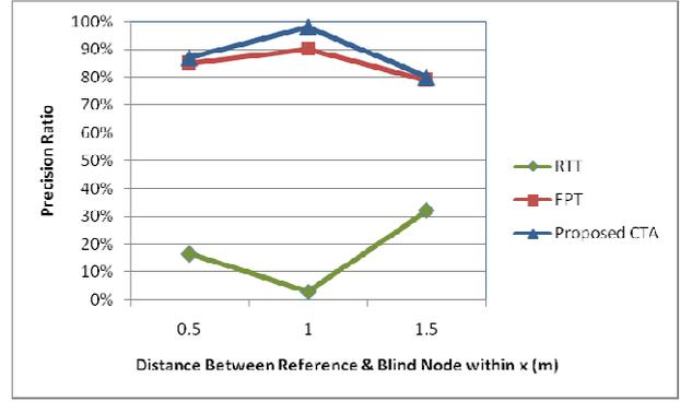
Fig. 7 Precision when error distance within 1.0 m
