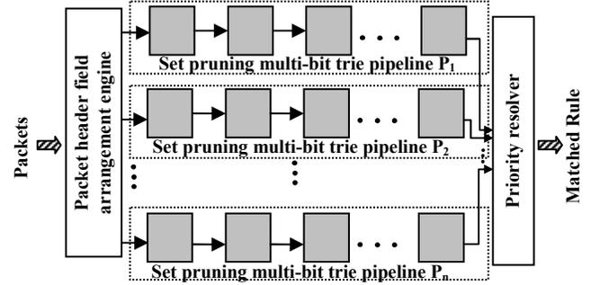
Figure 3. Block diagram of the parallel linear pipeline.
