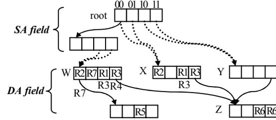
Figure 2. The 2-bit SPMT constructed from the rules in Table I.
