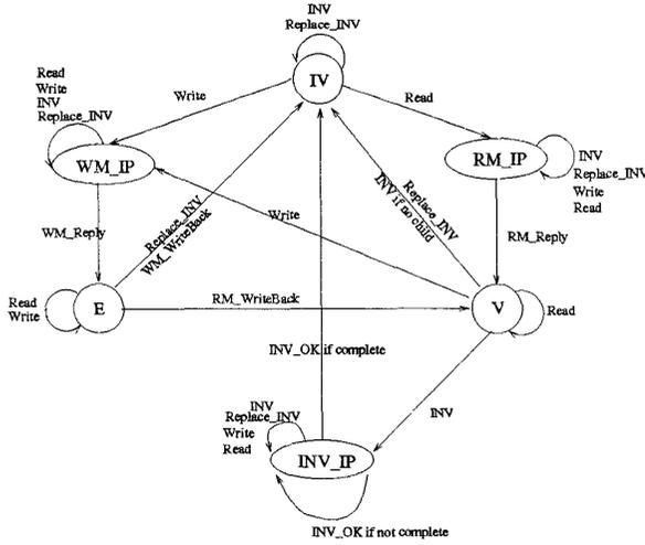
Figure 3: State transition diagram of the cache blocks.
