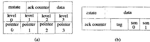
Figure 2: The structures of cache and memory blocks.
