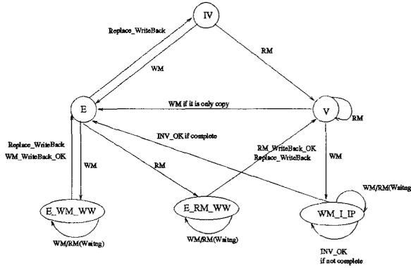
Figure 4: State transition diagram of the memory blocks.
