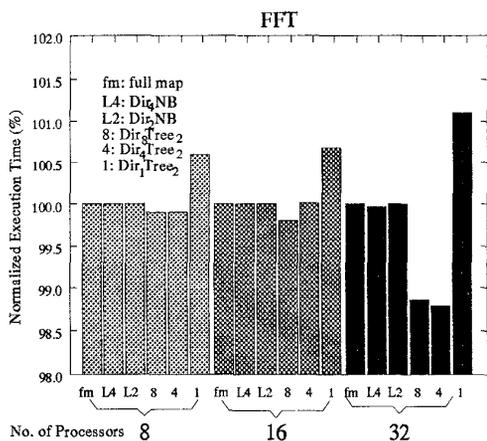
Figure 11: Normalized execution time for FFT.
