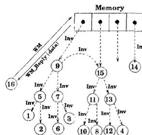
Figure 7: Message movements for a write miss. (For clarity, acknowledgments are omitted.)
