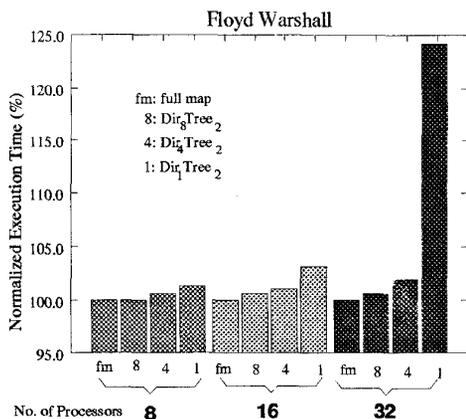
Figure 10: Normalized execution time for Floyd Washall.
