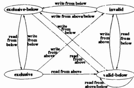
Figure 4: State transition diagram for a directory entry.
