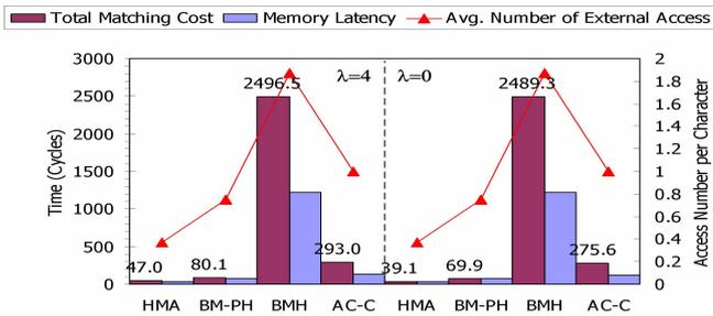
Fig. 4. The total processing time ( $\Psi$ ), the memory latency ( $\psi_M$ ), and the average number of external memory access ( $N_E$ ) for each input character, with  $\lambda = 4$  and  $\lambda = 0$  respectively.
