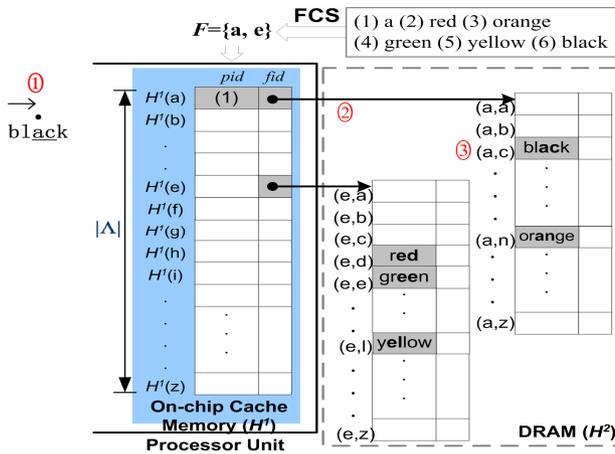
Fig. 2 The architecture of hierarchical hash tables.
