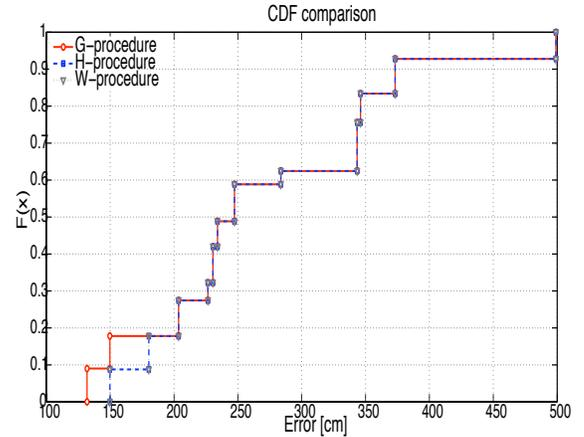
Fig. 5. Localization error using the Euclidean metric with the H, G, and W-procedures.
