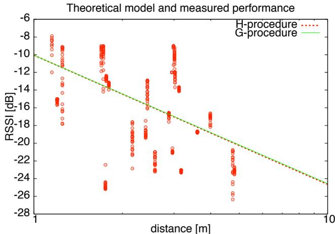
Fig. 2. Received RSSI measured from the mobile node.
