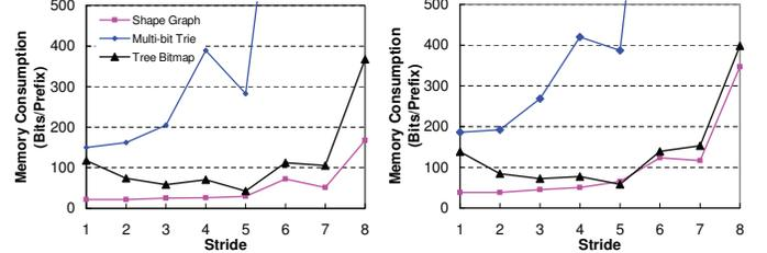
Fig. 10. Overall memory consumption comparison on two prefix tables. The left side is for AS1221 and the right side is for Maewest
