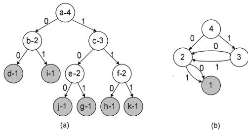
Fig. 4. Label the leaf-pushing trie with shape ids and build the shape graph
