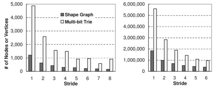
Fig. 13. The number of shape graph vertices vs. the number of multi-bit trie nodes for IPv6 forwarding tables. The left side is for the IPv6 BGP table and the right side is for the synthesized IPv6 table
