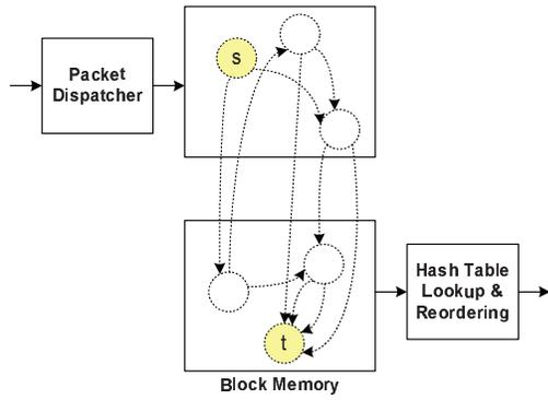
Fig. 8. Distribute graph vertices into multiple memory blocks to improve the lookup throughput.  $s$  is the starting vertex and  $t$  is the terminating vertex
