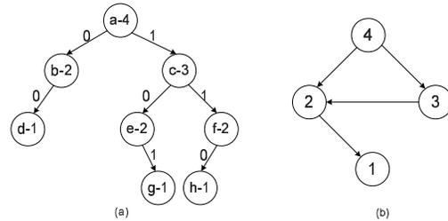
Fig. 2. Label the binary trie with isomorphic sub-tree ids and transform it to a directed graph
