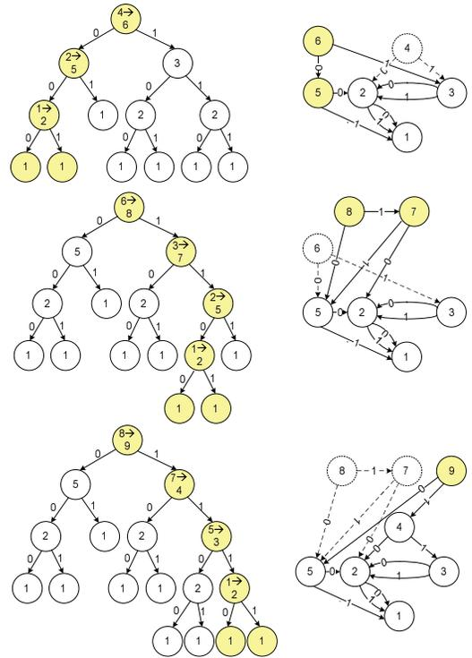
Fig. 7. Illustration of the shape graph updates as the new prefixes "001\*", "1100\*", and "1111\*" are inserted sequentially. Left side is the updated leaf-pushing binary trie and the right side is the updated shape graph. The dark nodes (vertices) indicate the newly inserted or updated nodes (vertices). The dashed vertices and edges in the shape graph indicate the unused vertices and edges after the update
