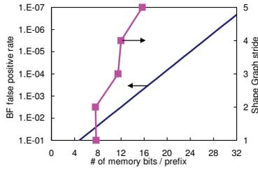
Fig. 11. On-chip memory consumption for different Bloom filter false positive rates and different shape graph strides. the memory consumption is normalized to bits per prefix.
