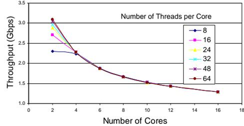
Figure 8. Performance of Multi-Core Architecture for Full-Text Search
