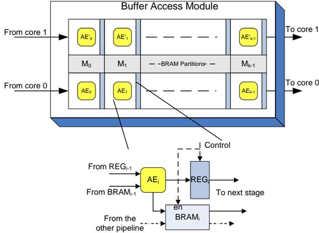
**Figure 6. BRAM Buffer Access Module**
