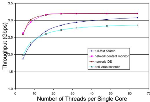
Figure 7. Throughput for a 2-Core System
