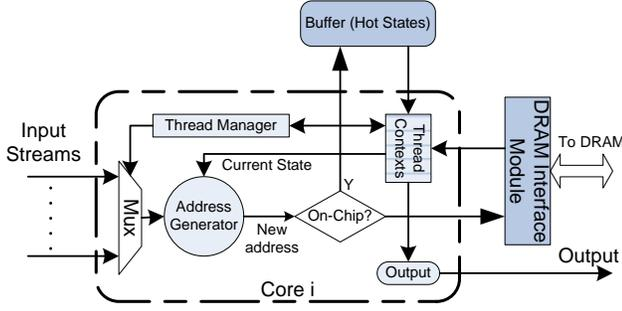
Figure 5. Structure of a Core
