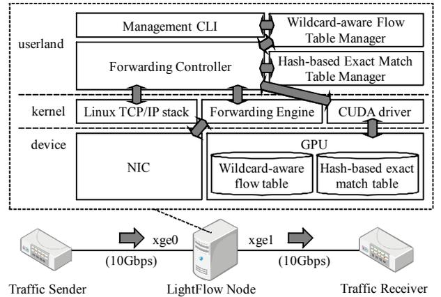
Figure 5. Setup for the demonstration.
