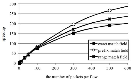
Figure 7. Speedup effect of wildcard-aware flow table coordinating with hash-based exact match table.
