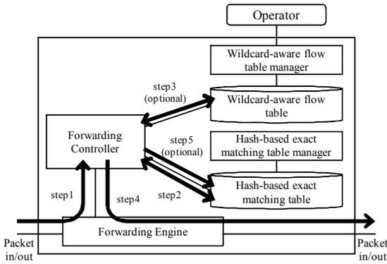
Figure 2. The LightFlow architecture.
