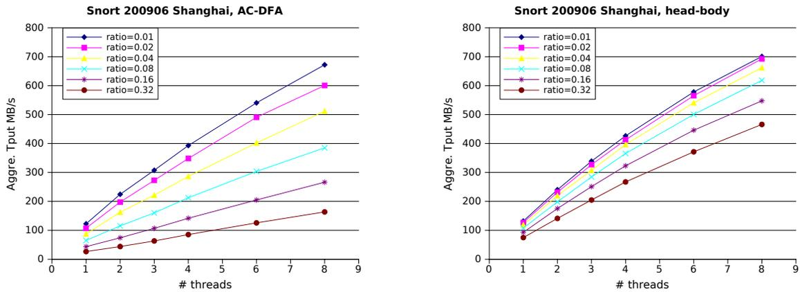
Figure 8. Aggregated throughput of AC-DFA (left) and HBM with 16,340 head states (right) for Snort0906 on Shanghai.
