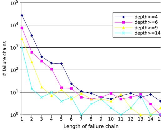
Figure 4. Number of failure chains versus length above various depth in Snort dictionary’s AC-DFA.
