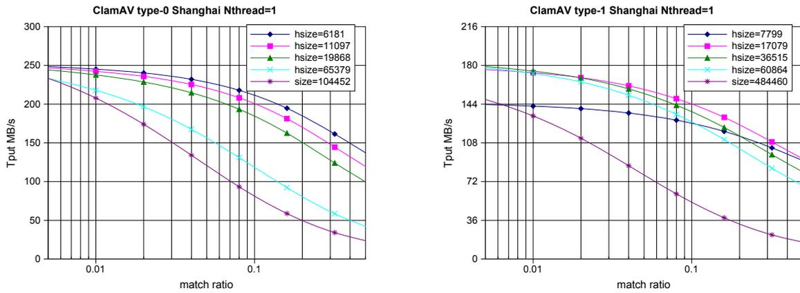
Figure 7. Throughput of AC-DFA and HBM with various head sizes for CAV-0 (left) and CAV-1 (right) on Shanghai.
