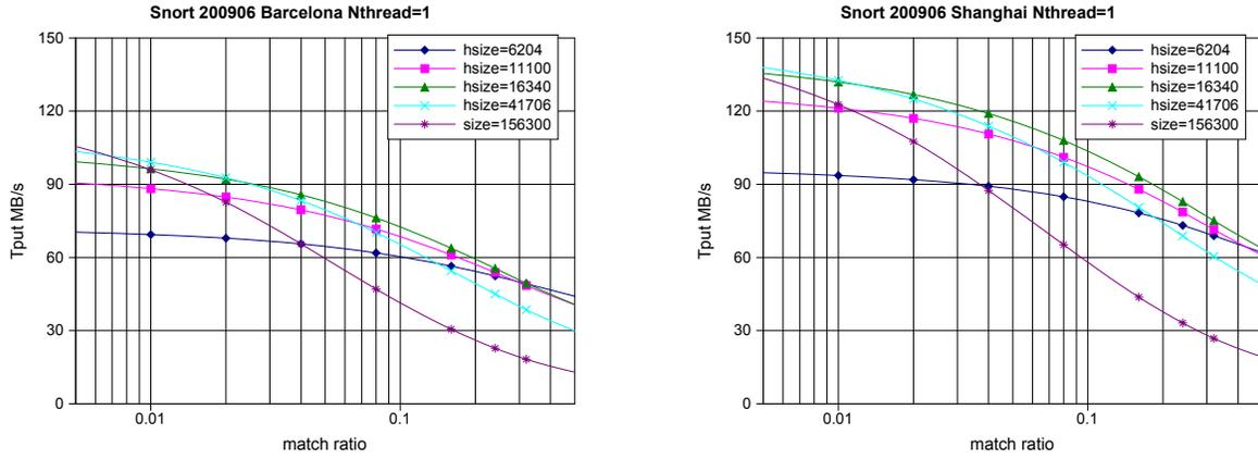
Figure 6. Throughput of AC-DFA and HBM with various head sizes for Snort0906 on Barcelona (left) and Shanghai (right).
