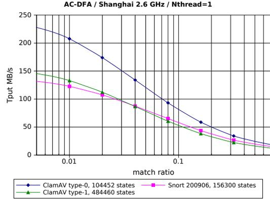
Figure 1. Single-threaded throughput of fully populated AC-DFA vs. match ratio on 2.6 GHz AMD Opteron processor (Shanghai).
