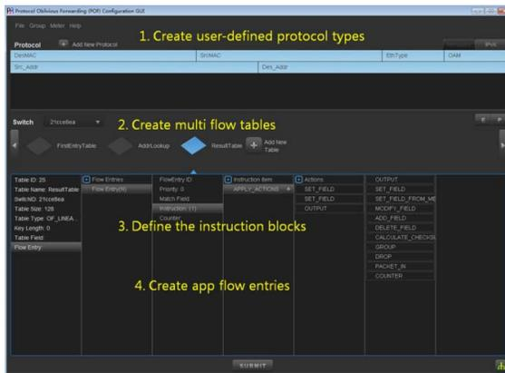
Fig. 5. GUI of POF Controller.
