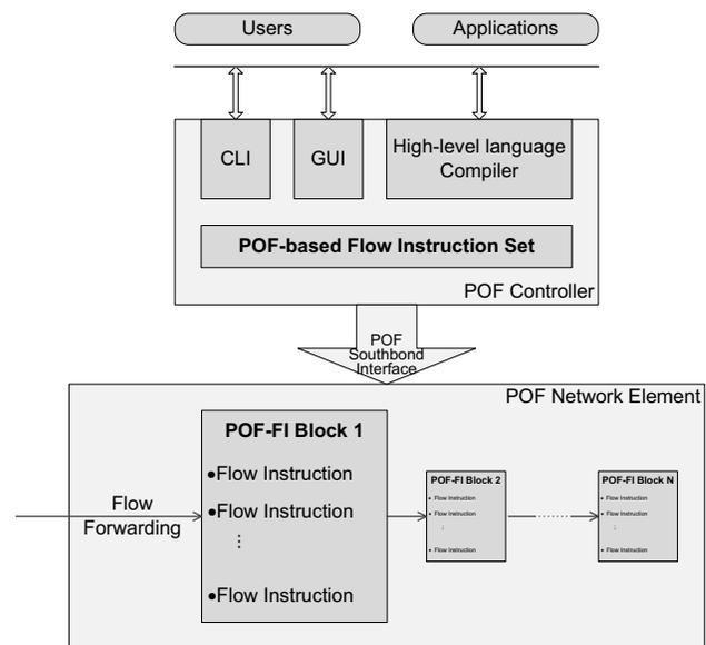
Fig. 1. The position of POF-based Flow Instruction Set in POF framework.
