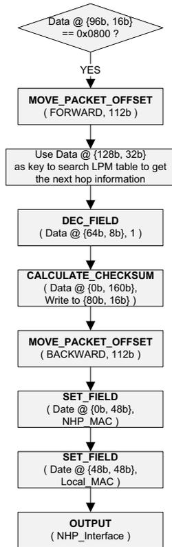
Fig. 4. How to handle the Ethernet and IPv4.
