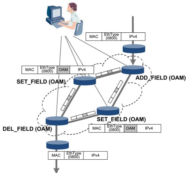
Fig. 2. Usage of POF-FIS in users' LAN with the custom OAM field.
