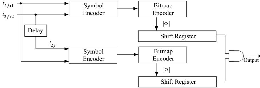
Fig. 9. The structure of a high throughput module circuit processing two characters at a time ( $q = 2$ ) with the bitmap encoder.
