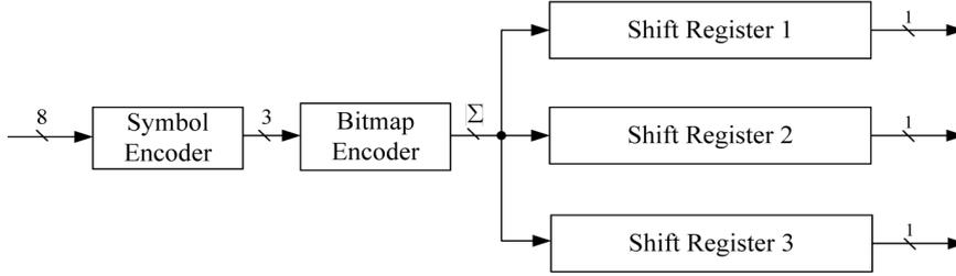
Fig. 8. The sharing of the same symbol encoder and bitmap encoder by three different Snort rules. Each character is also assumed to be an ASCII. All the Snort rules use the same alphabet comprised of 7 symbols.
