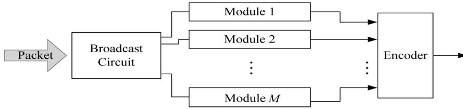
Fig. 2. The basic structure of the proposed circuit, where  $M$  is the number of rules implemented by the circuit.
