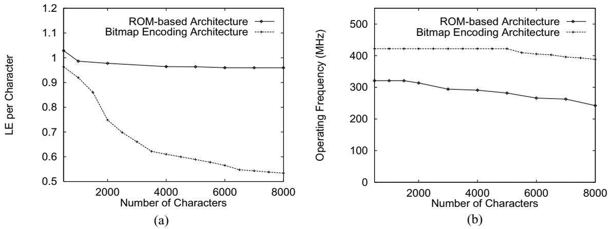
Fig. 10. The performance of the ROM-based and bitmap encoding circuit with  $q = 1$  for various rule sets sizes ranging from 500 characters to 8000 characters (a) LE per character (b) Operating Frequency.
