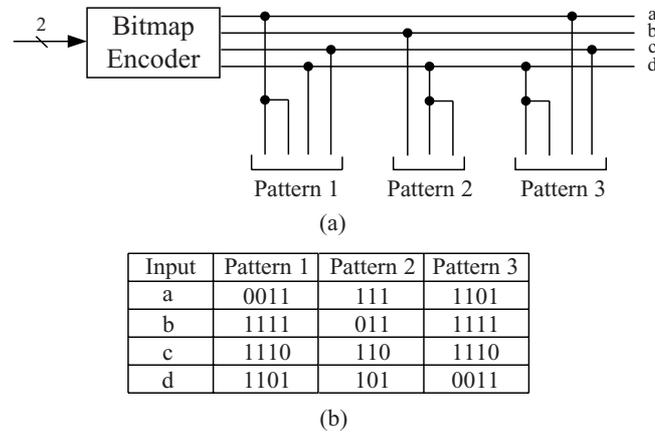
Fig. 6. An example of three patterns (*aadc, bdd* and *ddac*) share the same bitmap encoder, (a)The architecture (b)Table of three patterns.
