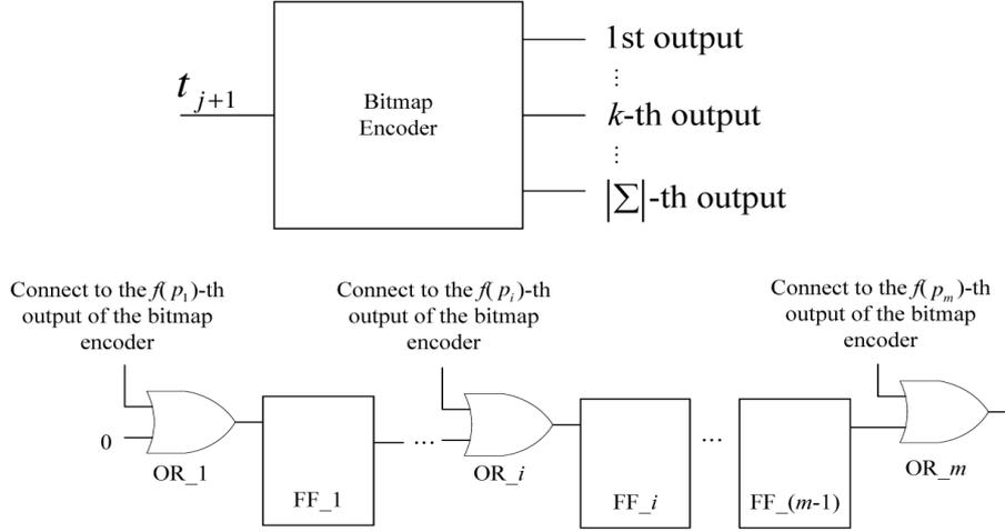
Fig. 4. The shift-or circuit based on a bitmap encoder.
