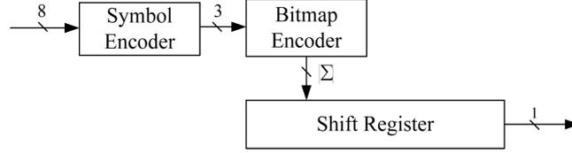
Fig. 7. The increase of a symbol encoder for reducing the bitmap encoder size. In this example, each input character is assumed to be an ASCII code (8 bits). We also assume the Snort rule uses only 7 symbols in the alphabet. The output of the symbol encoder is 3 bits.
