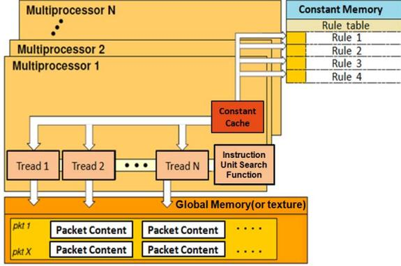
Figure 3. The use of memory on CUDA device.
