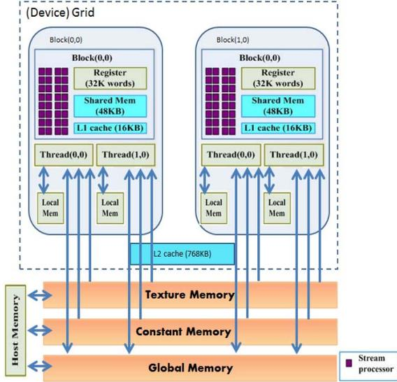
Figure 1. Memory architectures of CUDA device.
