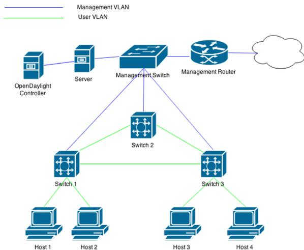
Fig. 1. Network topology used for testbed and Mininet
