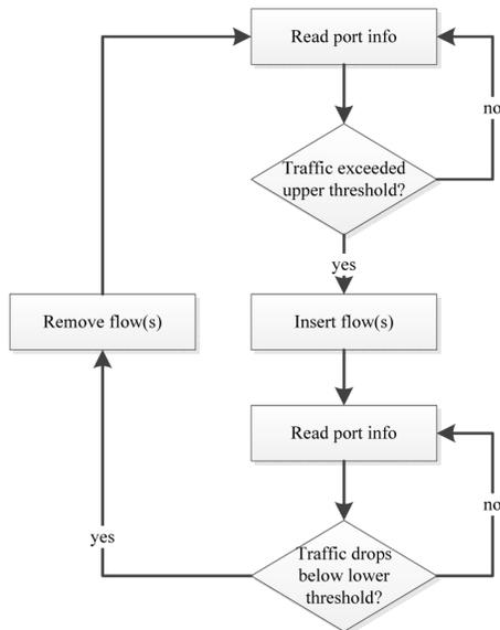
Fig. 4. Flowchart of the dynamic traffic diversion application
