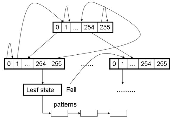
Figure 2. The ClamAV trie structure.
