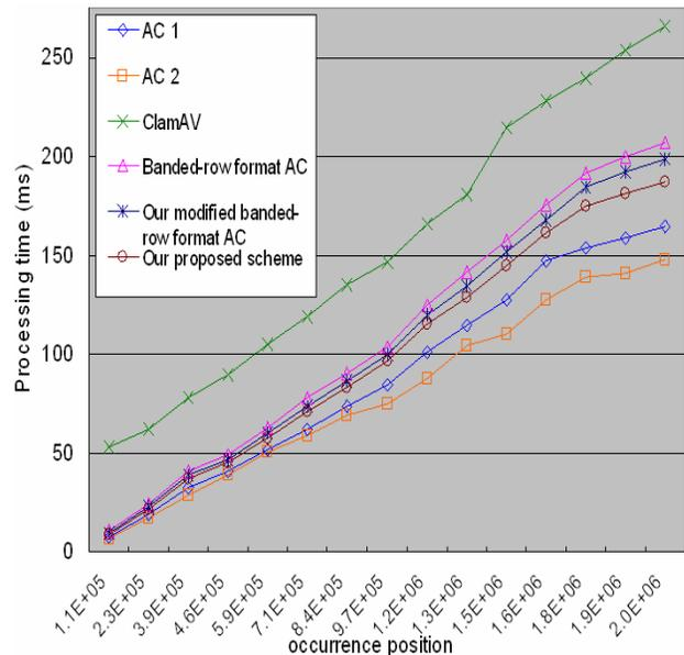
Figure 6. Processing time comparison for scanning a file with a pattern occurrence.
