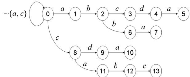
Figure 3. The goto function for  $\Sigma = \{a, b, c, d, e, f, g, h\}$  and  $Y = \{abcd, abba, cda, cab\}$ .
