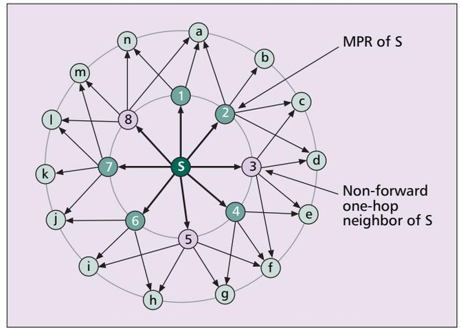
Figure 4. Minimum overlapping MPR heuristic.
