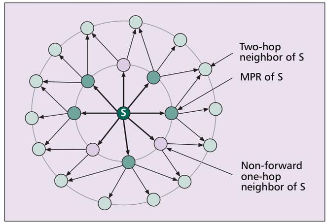
■ Figure 2. MPR flooding heuristic.
