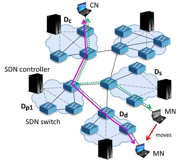
Fig. 1: Overview of SDN based mobility management architecture
