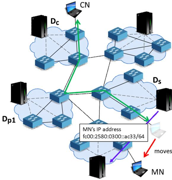
Fig. 2: Transmitting IP address after movement of MN
