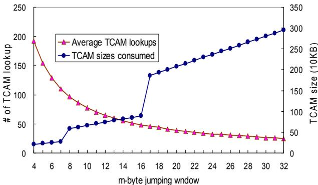
Fig. 8. The number of TCAM lookups and the size of TCAM in  $m$ -byte jumping window
