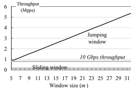
Fig. 6. Packet inspection throughput of jumping and sliding windows
