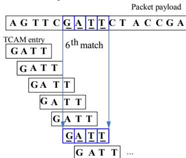
Fig. 1. TCAM-based packet inspection with “sliding window”
