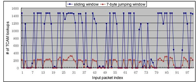
Fig. 9. The simulation result of TCAM lookups for packet trace
