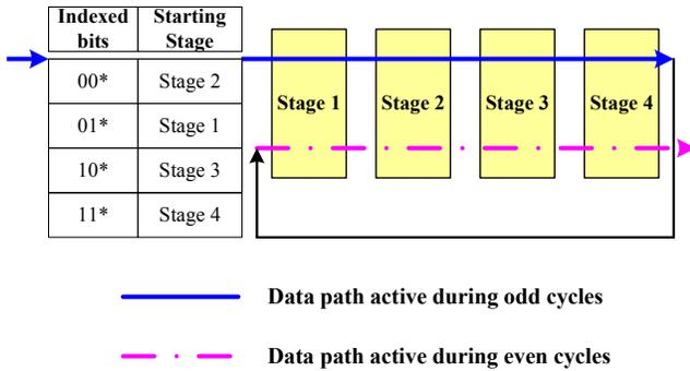
**Figure 2. Example of Ring pipeline architecture [1].**
