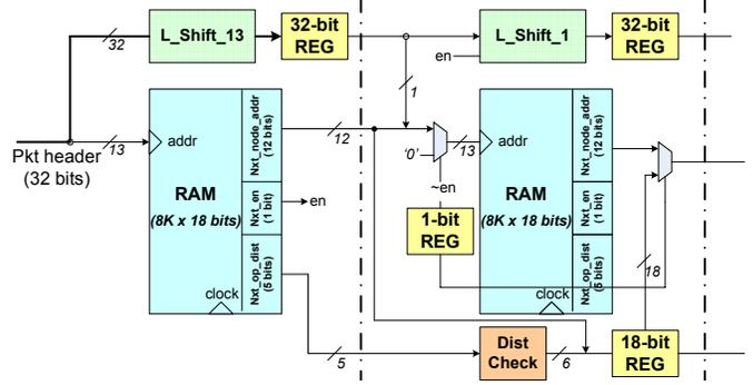
**Figure 6. OLP schematic for FPGA implementation.**
