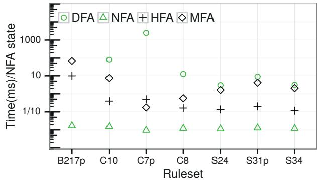
Fig. 3: Construction times for DFA, HFA, NFA and MFA
