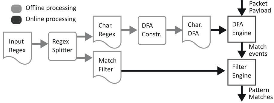
Fig. 1: Match filter generation and use
