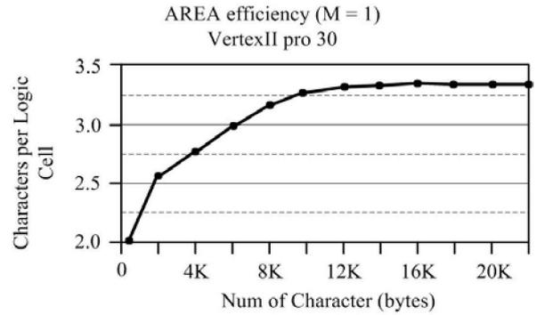
Figure 8, area efficiency analysis of HBC based pattern matching implementation. The parallelism parameter  $M = 1$ . With the increasing of matched characters, the matched characters of a logic cell will increase. The Max area efficiency will in crease to 3.13 matched characters per logic cell when implementing all the SNORT v2.0 rules.
