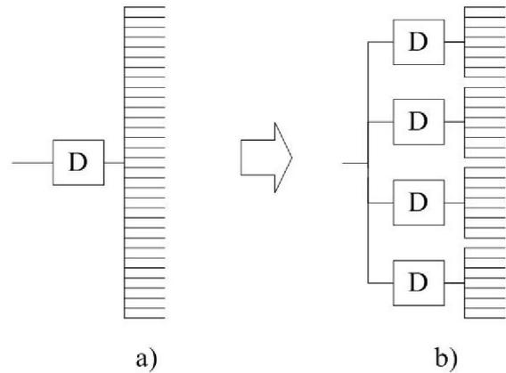
Figure 4, Using registers to solve the large numbers of fan out problem. A register with 32 fan outs in a) can be replaced by 4 registers with 8 fan outs in b).
