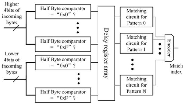
Figure 2, Using HBCs to implement all the SNORT Rules, There are total 32 HBCs, the output of delay register array is shared. Every pattern has a dedicated matching circuit. The matching circuit connects the necessary delayed compare results as inputs.
