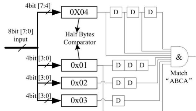
Figure 1, HBC architecture for pattern "ABCA" matching. The output of comparator for 0x04 is shared in comparing the higher 4 bits for all the 4 characters. The output of comparator for 0x01 is shared in comparing lower 4 bits for the first and last character "A".
