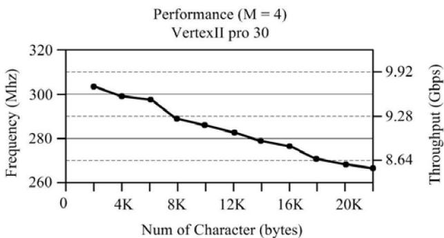
Figure7, performance analysis of HBC based pattern matching implementation. The parallelism parameter  $M = 4$ . The system clock can be 268 Mhz when implement all the SNORT v2.0 rules. And the max throughput is 8.576Gbps.
