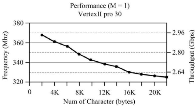
Figure 6, performance analysis of HBC based pattern matching implementation. The parallelism factor  $M = 1$ . The max system clock is 325 Mhz when implement all the SNORT v2.0 rules (more than 22,000 characters). And the max throughput is 2.6Gbps.
