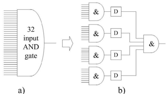
Figure 5, Using registers to the huge combination logic. 32 inputs AND gate in a) can be divided into two groups of small AND gate (8 inputs and 4 inputs) which separated by registers in b).
