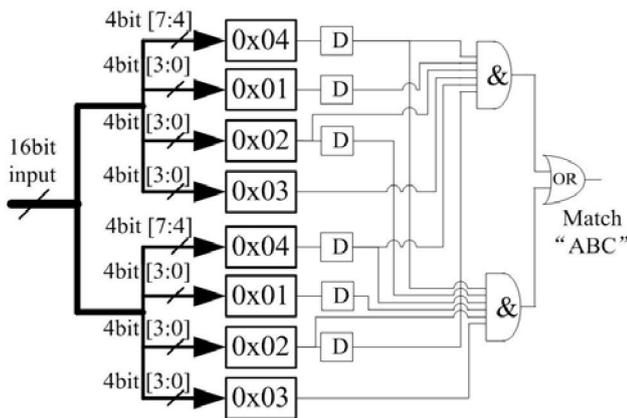
Figure 3, Doubled HBC groups process 2 input bytes per cycle. The start character of the predefined matching pattern may occur at the higher byte or lower byte of the input parallel two bytes
