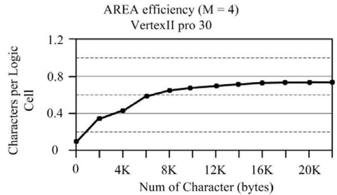
Figure 9, area efficiency analysis of HBC based pattern matching implementation. The parallelism factor  $M = 4$ . The max area efficiency is 0.71matched characters per logic cell.
