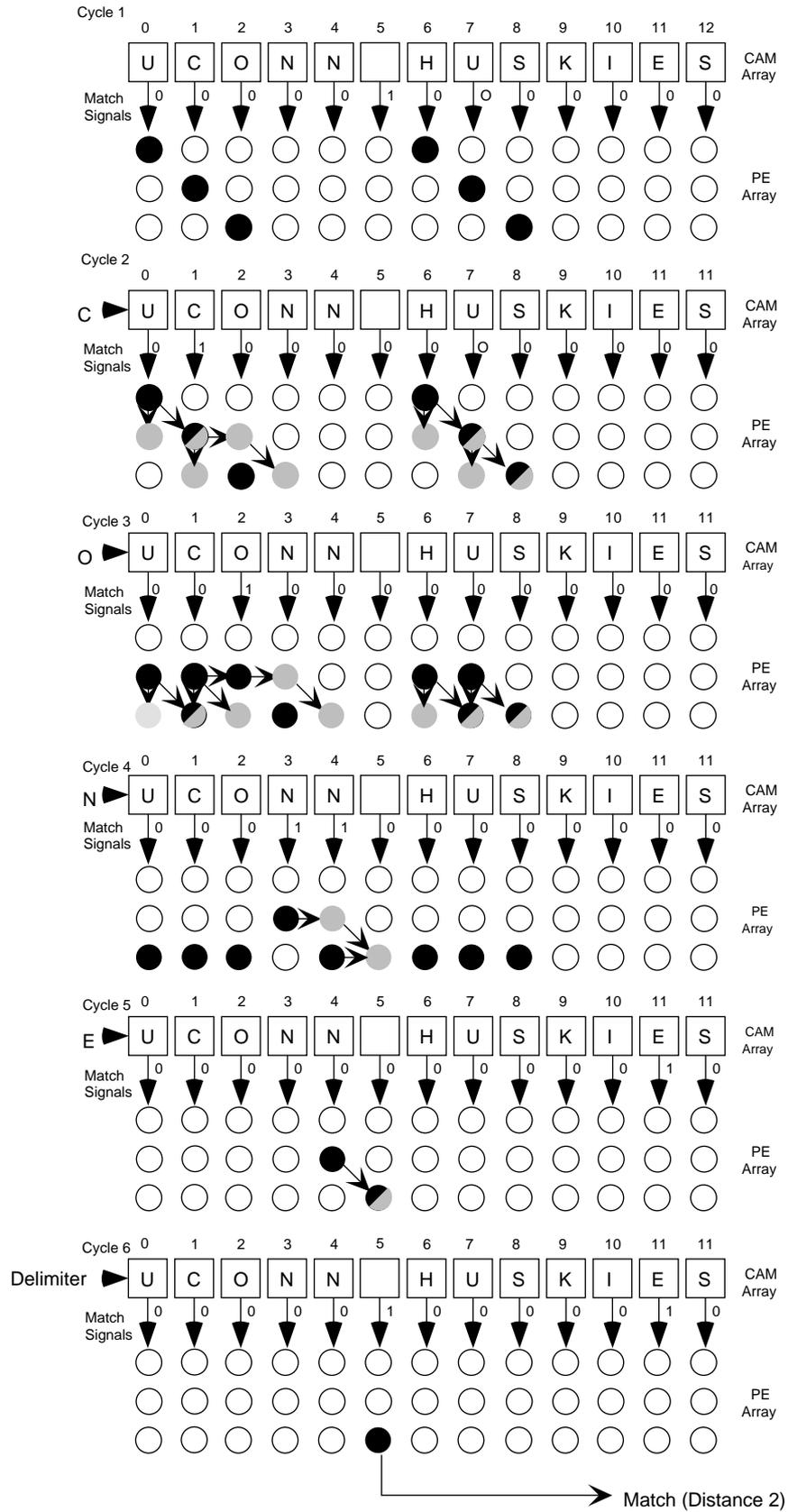
Fig. 6. Keyword match processor example.
