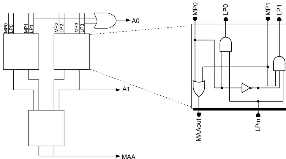
Fig. 5. MAO logic binary tree (four bit example).
