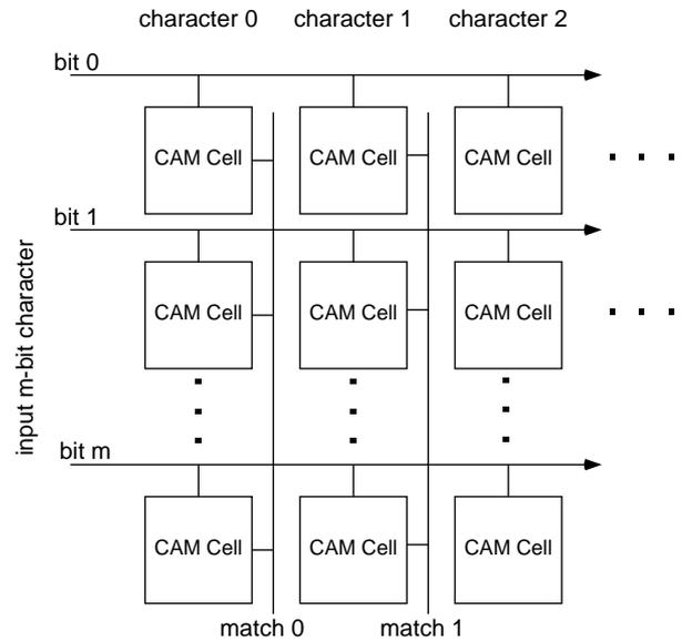
Fig. 3. CAM array.
