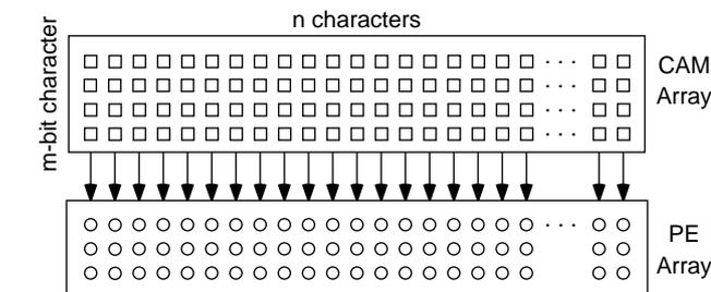
Fig. 2. CAM and PE array layout.
