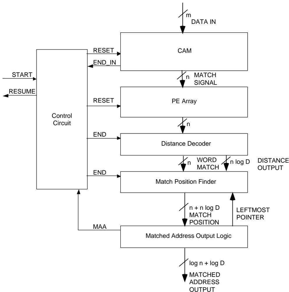
Fig. 1. Keyword match processor architecture.
