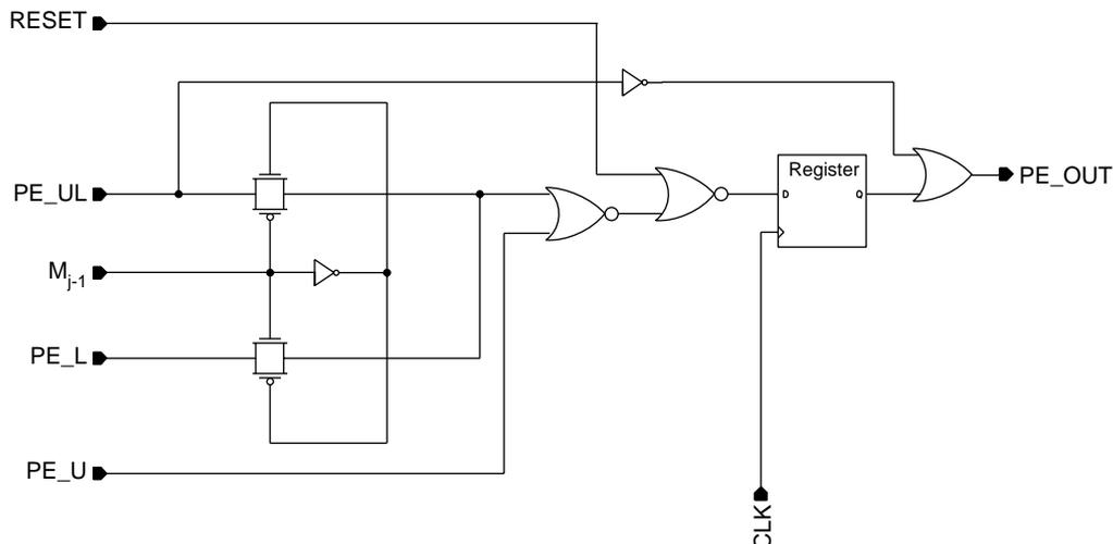
Fig. 4. Keyword match processor PE design.
