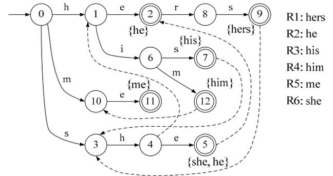
Figure 2. AC automaton for rule set {hers, he, his, him, me, she}. For simplicity, failure transitions to the root state are not shown.
