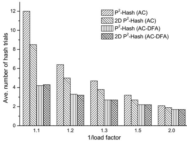
Figure 7. Average number of hash trials required for each transition placement under Snort rule set
